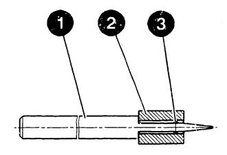
Tool for pressing out needle bearing in armature
